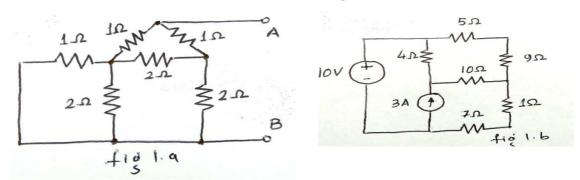
b. Using mesh current analysis finds loop currents for the circuit shown in fig (1.b).
