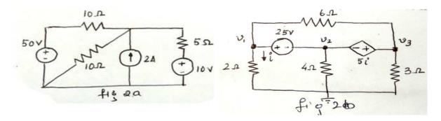
b. Find all node voltages for the circuit shown in fig (2.b) using node analysis.
